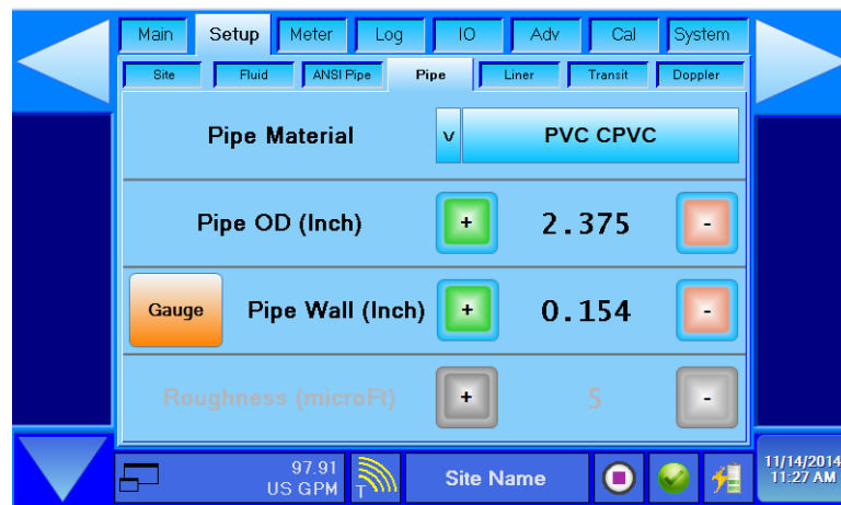
Figure 56: Setup &gt; Pipe
