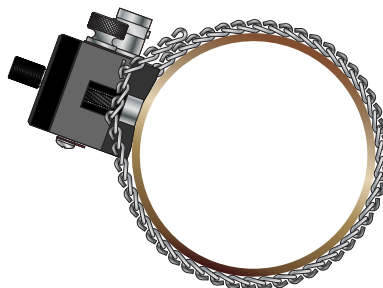
Figure 29: DTTSU transducers mounted
